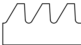
锯齿螺纹 buttress thread
