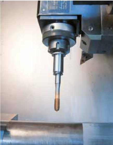
The new STA Synchro Tapping Adaptor was designed specifically for collet chucks and allows for synchronous thread cutting and forming to be used with all suitable machines.
